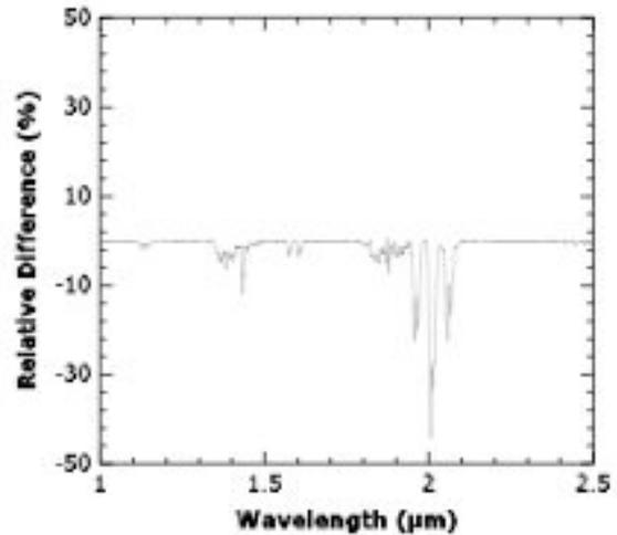
Figure 4 — Result of a simulation showing the errors introduced into a spectrum of Mars by using the “standard star” method to remove telluric absorption.
