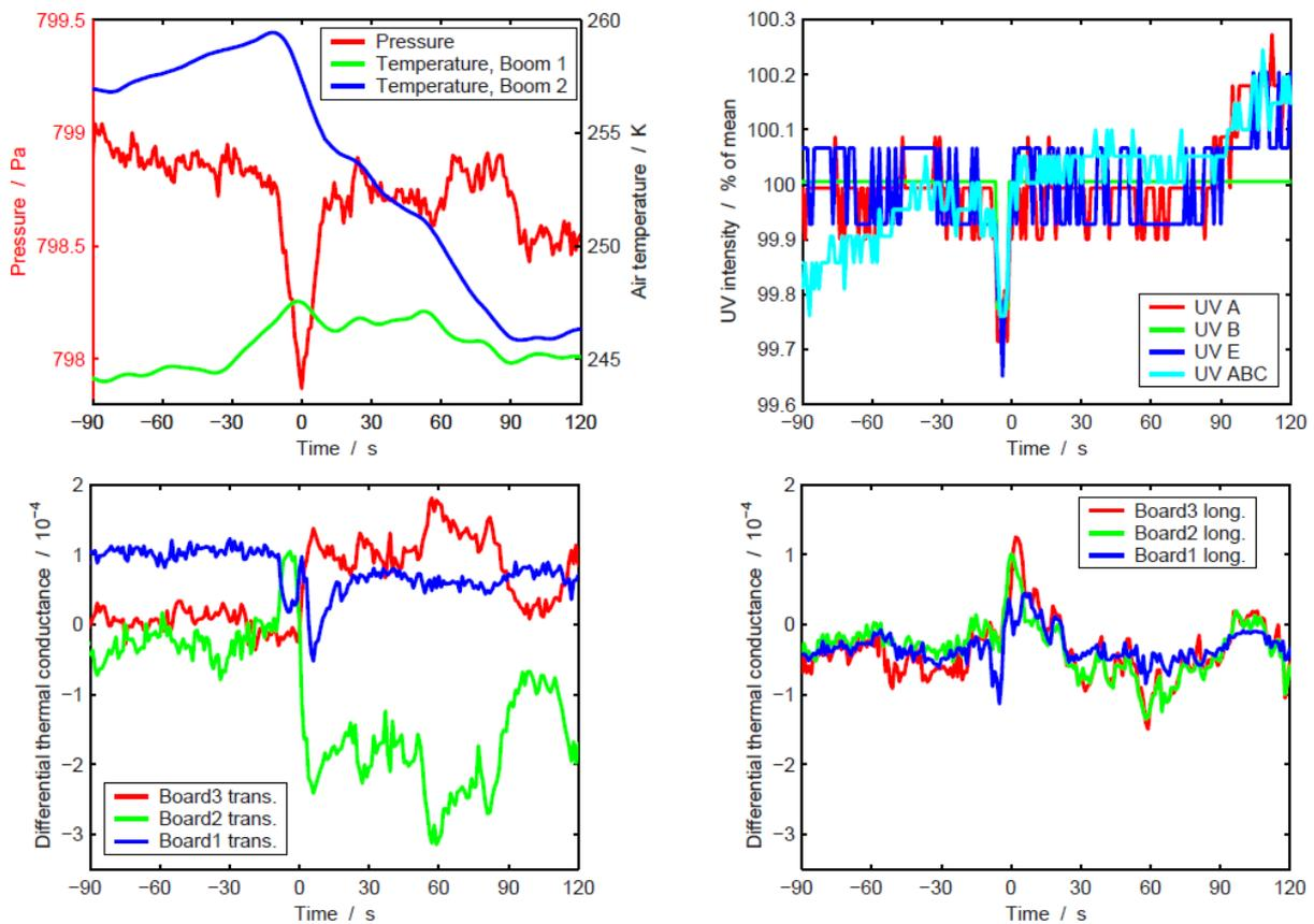
**Figure 1:** REMS measurements during a vortex event on MSL sol 86 at 11:02 Local Mean Solar Time. Top left: pressure and air temperature. Top right: Ultraviolet radiation intensity. Bottom left: wind sensor raw data in transversal direction. Bottom right: wind sensor raw data in longitudinal direction.
