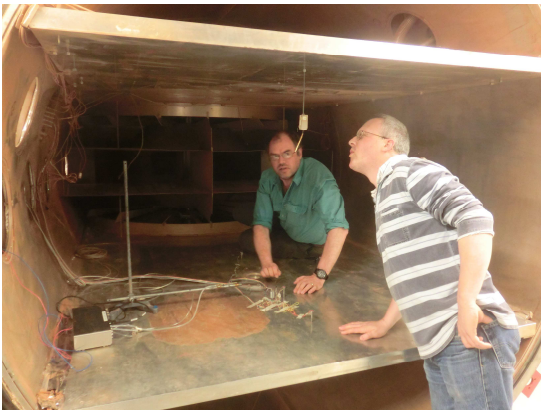
Figure 3. Installing microphones on the floor of the tunnel working section, near a pitot tube to independently measure pressure fluctuations. A telltale wind indicator hangs from the tunnel ceiling, and the fans that drive the wind are visible at the back.
