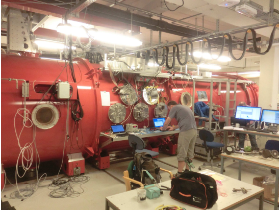
Figure 2. The Aarhus Chamber. As well as rapid (<1 hr) pump down to Mars pressure, the facility has many windows and feedthroughs to monitor conditions insides and permits rapid experiment reconfiguration.
