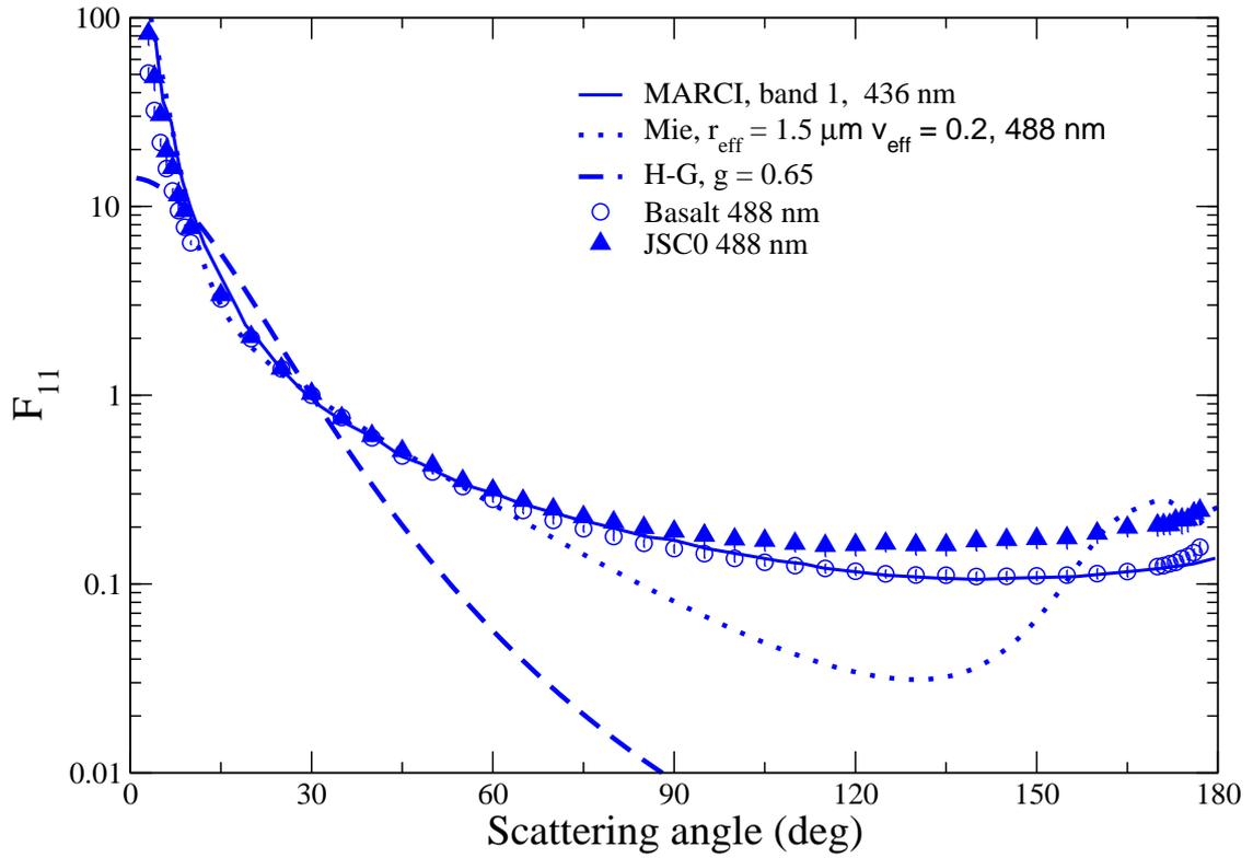
Figure 2: Pseudo Emission Phase Function constructed from MARCI band 1 (Wolff et al. 2010) at 436 nm (solid line) (top). We also present the analytical Henyey-Greenstein phase function for  $g=0.65$  (dashed line), and calculated phase functions for spheres (dotted line) together with our measurements for basalt, and JSC0 samples at 488 nm. After Dabrowska et al. 2015.
