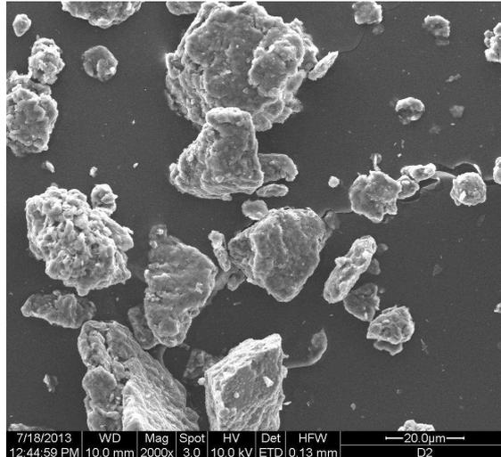
Figure 1: Scanning Electron Microscope images of montmorillonite. White bar denotes the scale of the image.
