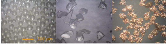
Fig.1: The three materials used in the study: glass spheres, quartz particles and copper particles. All particles were in the size range \sim 100 - 125 \mu\text{m} after being sorted through sieving.
