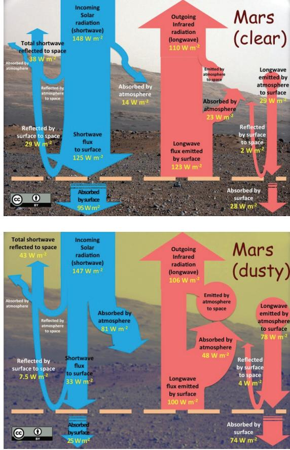
Figure 2: Schematic global radiative energy budgets for Mars, using data from the Mars Climate Database [4] and computations from NEMESIS [7]. Upper frame shows exchanges prevailing under normal (low dust optical depth;  $\tau = 0.3$ ) conditions, while the lower frame shows exchanges when the dust optical depth is up to  $\tau = 5$ .
