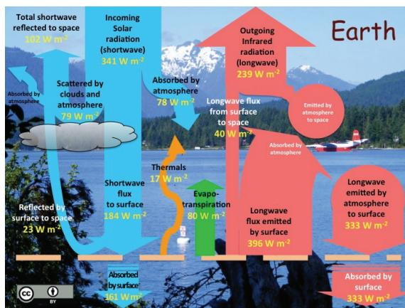
Figure 1: Schematic global energy budget for the Earth, using data obtained by Trenberth et al. [1].
