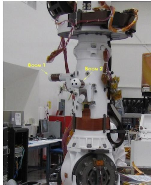
Figure 1: Remote Sensor Mast with the Boom 1 (B1) and Boom 2 (B2) installed. B2 is looking forward and B1 is pointing to the rover right side. At the beginning of the project, the minimum distance to the rover body and RSM head was estimated with the help of a quite simple CFD model. Also, the rover design has a constraint to minimize the size of any protrusion close to the booms.
