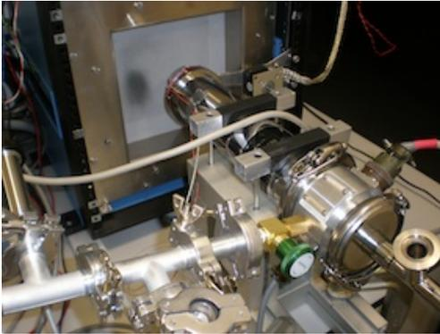
Figure 3: GTS set up for sensor calibration. The main GTS calibration has been carried with the help of a cryostat and a blackbody. Inside the cryostat were reproduced the operational conditions on Mars: low temperature, low pressure and carbon dioxide atmosphere. The black body placed in front of the sensor was the infrared radiation reference.
