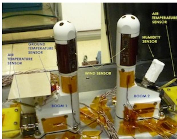
Figure 2: Boom 1 and 2 during the TVT tests. Some calibration tests have been run during TVT. One of them related with the GTS, reason by what a small plate has been place in front of the GTS in order to control the infrared radiation received by it. Regarding the WS, TVT had been used to determine its thermal conductivity losses.
