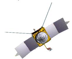
Artist's rendition of the MAVEN spacecraft in its on-orbit configuration. Instruments are mounted on the body, on the extensions at the end of the solar arrays, on three booms on the top of the spacecraft, and on an articulated payload platform on the bottom. The body-mounted high-gain antenna, seen in the middle, is 2 m across.
