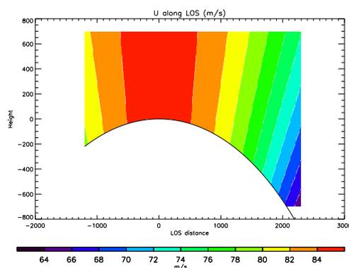
Figure 4: 2-D cross section of the winds projected along the line of sight in our problem, for an idealized constant zonal wind of 85 m/s. As in Figure 2, the viewing direction coincides with the lines of sight. The shape of Mars looks distorted due to the focus in the vertical scale. The wind value is maximum and equal to the zonal wind exactly at the limb (red area). See text.
