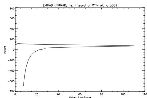
Figure 3: Simulation of the radiance emitted along the line of sight, obtained for a particular 1-D reference profile of the Martian atmosphere, extracted from the MCD. The vertical axis is tangent altitude over the planet; negative values for nadir pointing (see Figure 1). The maximum is obtained for a tangent altitude around 75 km.
