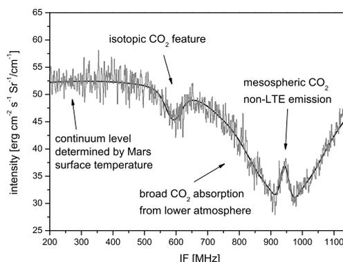
Figure 2: A typical spectrum of absorption and emission features of the P(2)  $\text{CO}_2$  transition to retrieve Doppler-shifted wind velocities on Mars. In black the best fit of a full atmospheric radiative transfer model to the spectrum is shown.
