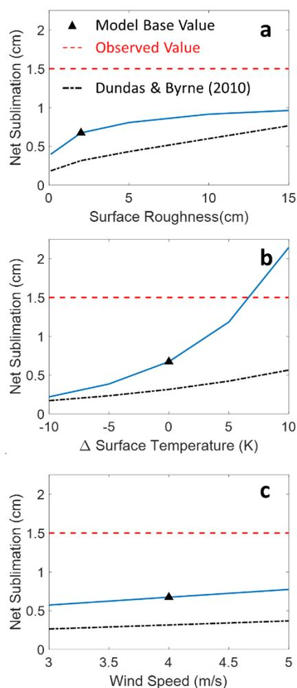
**Figure 3.** Sensitivity of the net sublimation (blue curves) over the four sols during which the 1.5-2 cm clods disappeared (dashed red lines) to: a) surface roughness, b) the simulated surface temperature relative to the base value and c) the wind speed at 2 m. The predictions of [1] for the same inputs are shown as black dashed lines for comparison.
