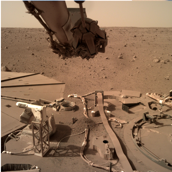
Figure 3: InSight on Mars. Dust everywhere Loads of dust particles on the deck and solar panels. Nevertheless, not any dust devil spotted in the whole mission. IDC image on sol 1211, April 24, 2022 at local time 2PM. NASA/JPL-Caltech.
