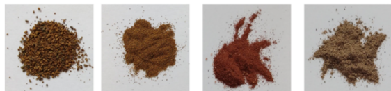
Figure 1 Martian dust analogues from left to right: JSC1-Mars < 1 mm, JSC1-Mars < 250 μm, MMS-2 and MGS-1.
