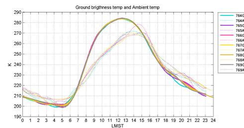
Figure 4. Typical evolution along several sols of ground and air temperatures (MSL kept its position in this period). Typically the maximum temperatures of ground and air are shifted by 2 hours and usually the air minimum is higher than the ground one.
