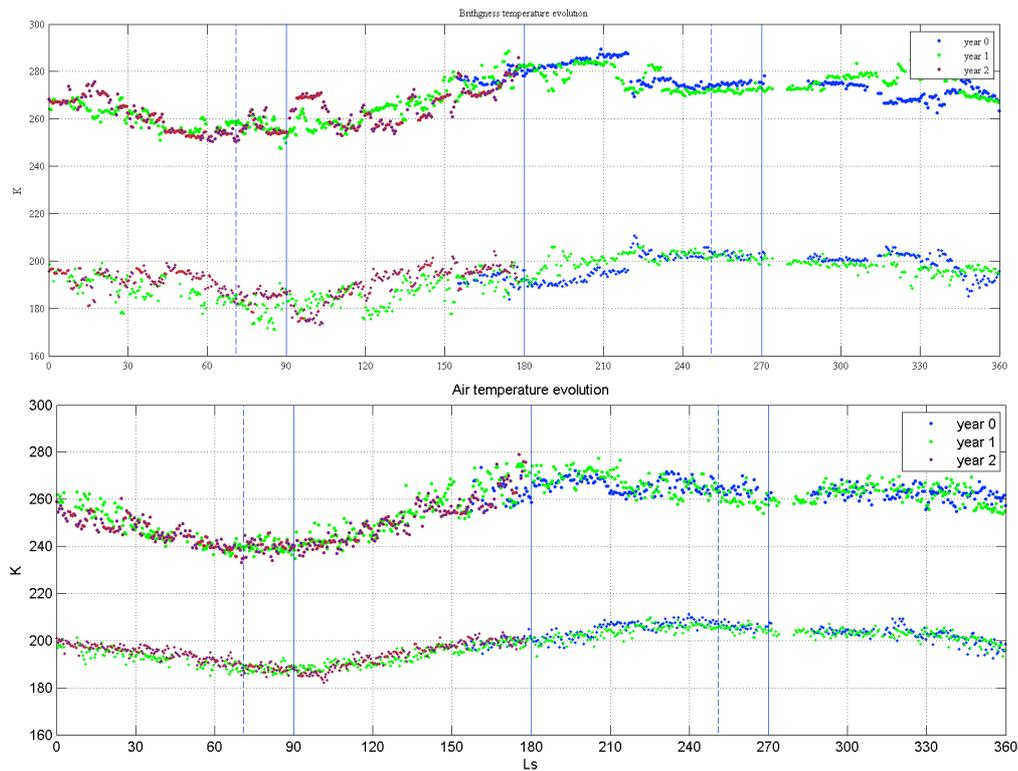
Figure 3. Ground brightness temperature (top) and air temperature (bottom). The Ground Temperature and Air Temperature sensors are quite dependent of the noise generated by the conditioning electronics, mainly during night. To mitigate this issue the values have been fitted by a Fourier serie of 8 terms and with a 1 sol period. The maximum and minimum values shown in the graphics correspond to those of the fitting curve.
