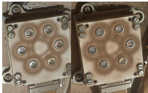
Figure 7. Images taken by MALHI on sols 660 (left) and 1041 (right). Independently of the different lighting conditions, it is clear that the amount of dust accumulated is growing with time. (Credit: NASA/JPL-Caltech/MSSSW)
