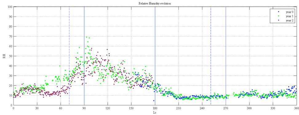
Figure 5. Humidity relative data .At each reading period, the data after the 3 first seconds is taken as representative for the full period. After that there is a self heating of the sensor and the values are not so reliable.
