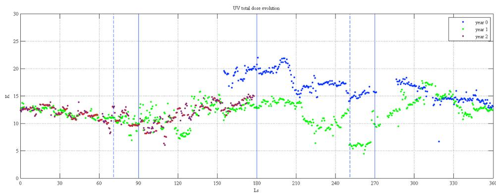
Figure 6. Ultraviolet total dose maximum readings. The dots values in the plot are the maximum reading each sol without any correction. This representation could be misleading because in many sols the UV field-of-view is blocked by the rover arm manipulator and unfortunately happen in most of the cases at the time of maximum irradiation, or is affected by the RSM shadow. Nevertheless, we believe that is enough to have a picture of the global evolution.
