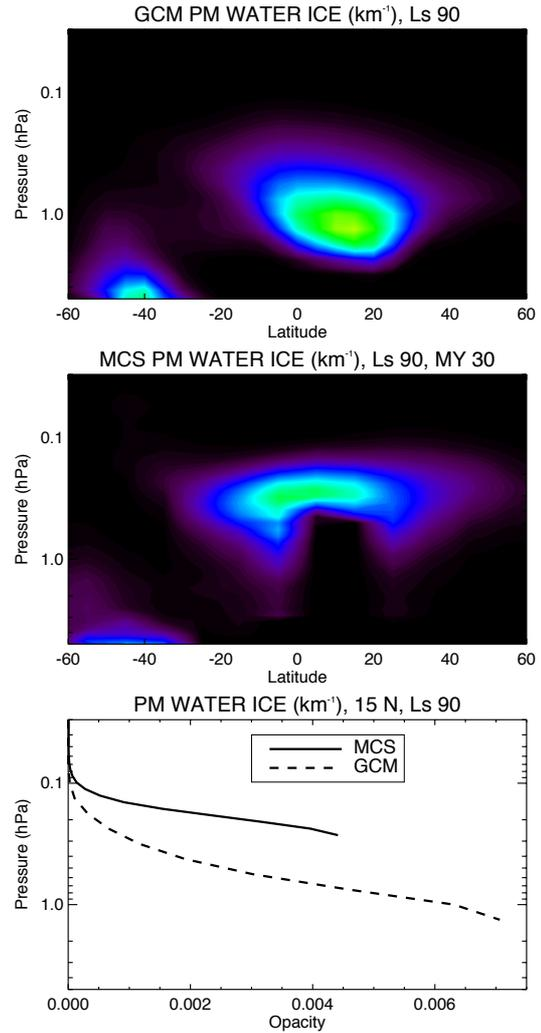
Figure 4: Zonal mean GCM-predicted (top) and MCS-observed (middle) water ice 12- $\mu\text{m}$  opacities at  $L_s$  90°. Profiles at 15 N (bottom).
