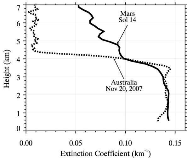
**Figure 2.** Profiles of extinction coefficient derived from the Phoenix Mars LIDAR measurements on mission sol 14. A profile measured above the Australian desert in windstorm conditions with an equivalent lidar system on 20 November 2007 (dashed) is shown for comparison.
