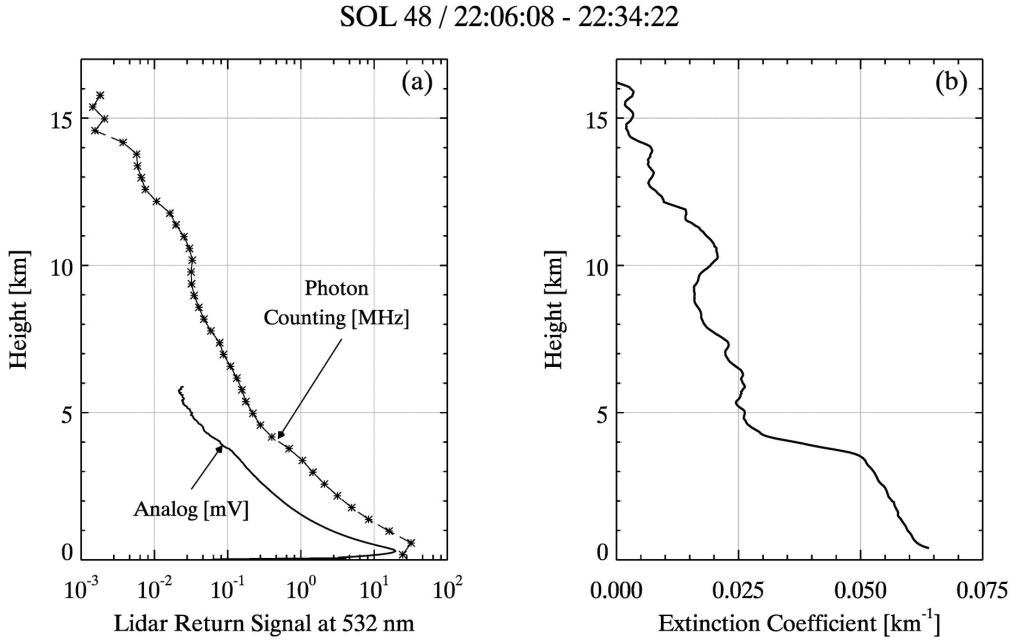
**Figure 1.** Phoenix LIDAR backscatter signal on mission sol 48 (a) and the derived extinction coefficient (b). There is greater atmospheric dust loading at heights below 4 km due to lifting from the surface and mixing within the Planetary Boundary Layer.
