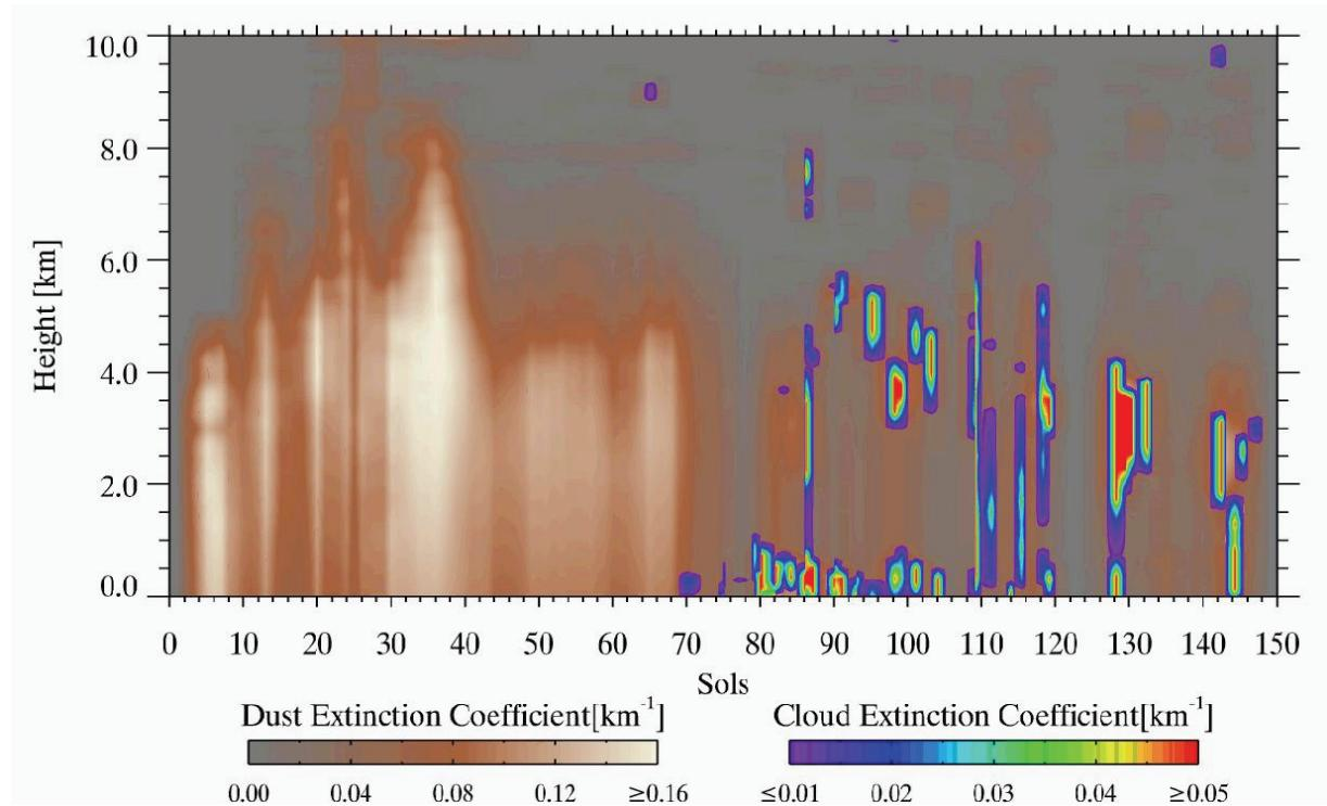
**Figure 3.** Contour plot of extinction coefficient derived from the Phoenix LIDAR measurements over the entire mission. The grey-brown-white colour scale is used for dust and the blue-green-red scale is used where clouds were detected. Gaps in the cloud contours over more than one day were due to a lack of nighttime measurements (e.g. sols 135-140).
